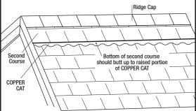
From left, use a roofing flat bar to lift bottom of 2nd course. Slide a COPPER CAT strip under 3/4" to where bottom of shingle butts up to COPPER CAT'S raised portion, nail down, repeat to end.
